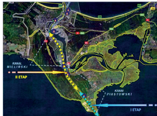
Figure 3. The stages of modernization (reconstruction) of Świnoujście-Szczecin channel (channels Piastowski and Mieleński) (UMS, 2009)
