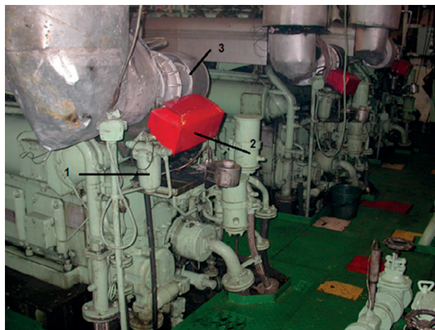
Figure 2. View of an auxiliary engine from side of the fuel filter on the ship from the series B-542: 1 – fuel filter, 2 – filter cover, 3 – turbocharger
