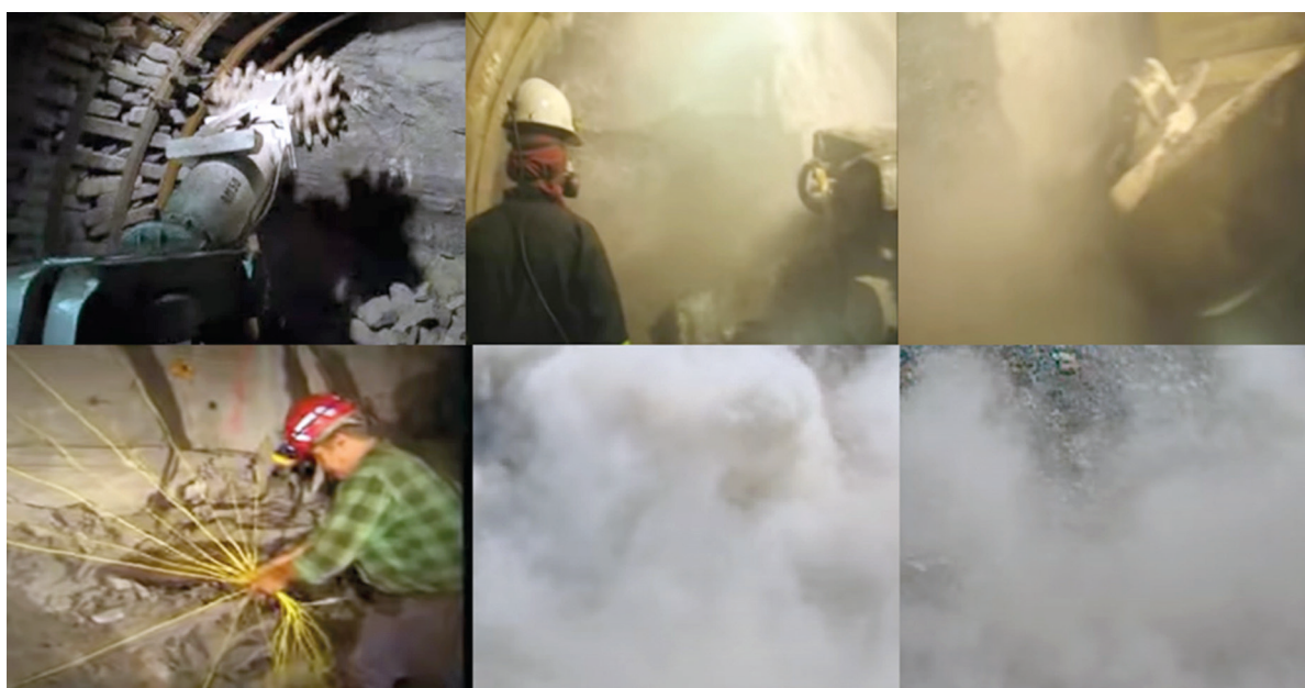
Figure 1. Dustiness during mine face works with the use of the AM-50 roadheader and explosives
